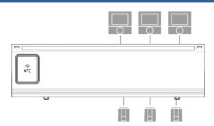
Parameters, settings and special functions can be changed or executed via the NFC app or Modbus interface. The set parameters and settings can be read out via NFC or the Modbus interface.
