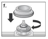
Screw the valve adapter manually onto the valve.
