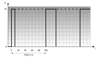
Pulse width frequency 100 Hz to 1000 Hz
